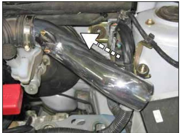
g. Insert the inlet pipe as shown.
