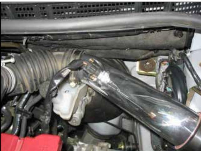
n. Plug in the MAF sensor connector.
