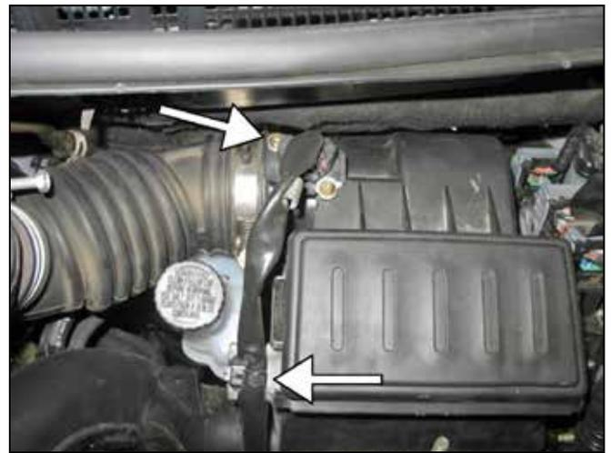
b. Unclip the Mass Air Flow (MAF) sensor wire harness connector and wire harness clip from the air box.
