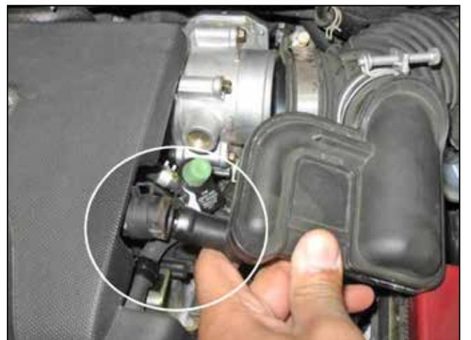
d. Unclasp the spring clamp for the crankcase breather tube. Remove the plastic resonator from the crankcase breather tube.
