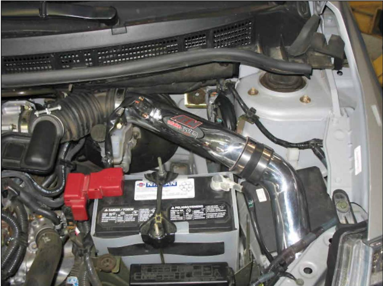
AEM® intake system installed
