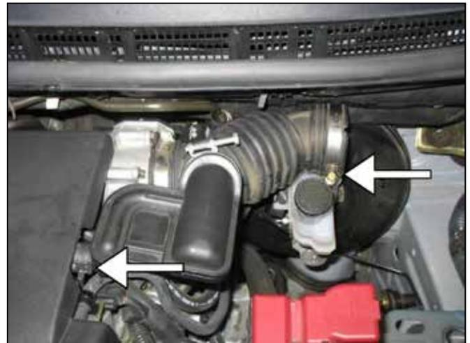
b. Insert the tree mount zip ties into the factory location on the battery bracket. Secure the ECU wire harness to the bracket. Cut off excess tie.
