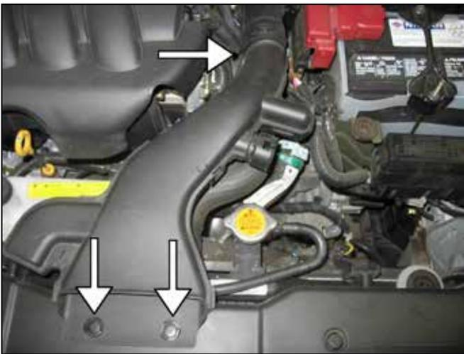
a. Remove the push-in tabs for the air inlet ducting. Unclip the air inlet ducting from the air inlet tube. Remove the air inlet ducting.
